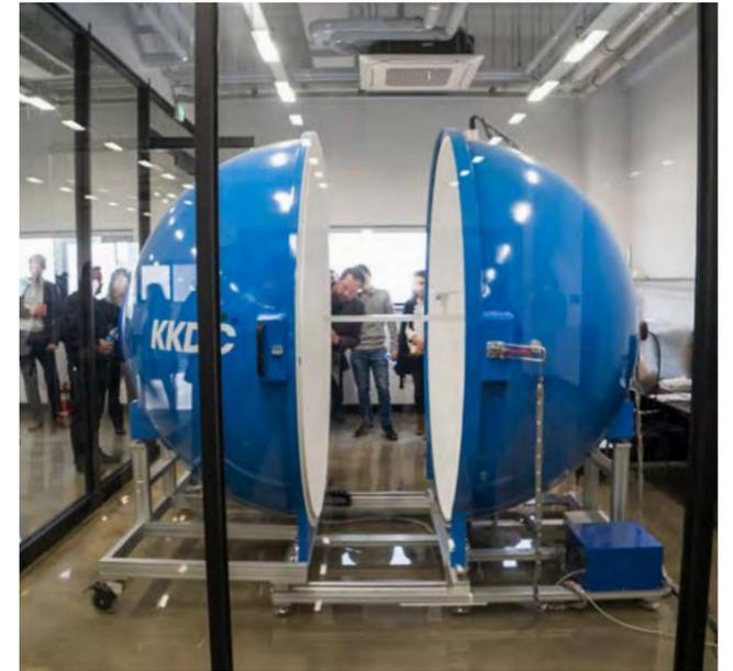
The in-house integration sphere ensures we can capture accurate luminaire output data to **certified LM-79 standard.**
